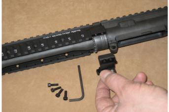
• Four 8-32 x <sup>1</sup>/<sub>2</sub> long Socket head cap screws. With Allen Key
